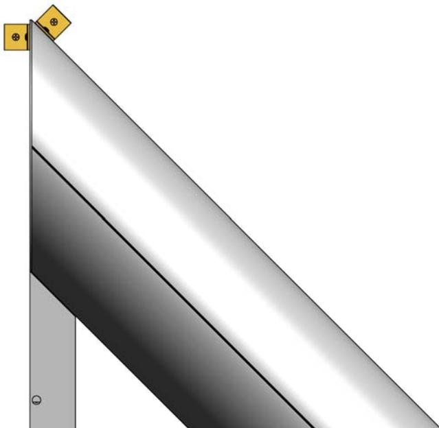
[EN] Please position the additional housing fixings as close to the top as possible. If this is not possible or cannot be done easily, carry out face mounting using the provided extra bracket. (->10.0) optionally try the possibility 11.0.
